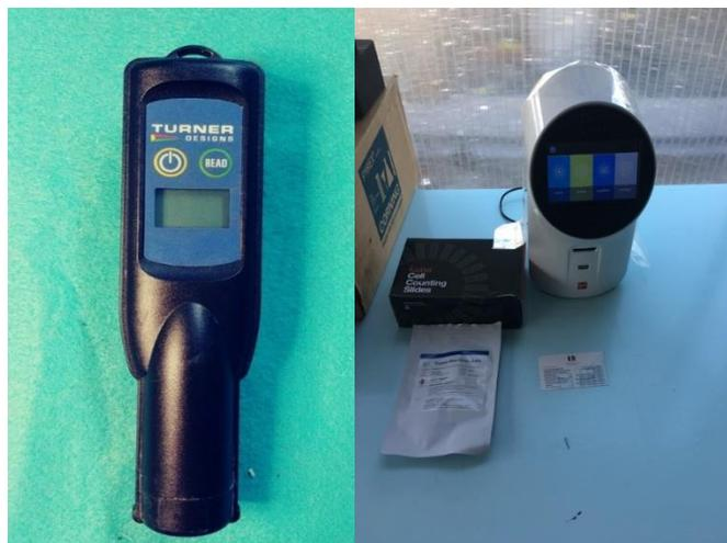
Figure 5. Turner Designs hand-held fluorometer (left) and Luna II Cell Counting Slide (right).
