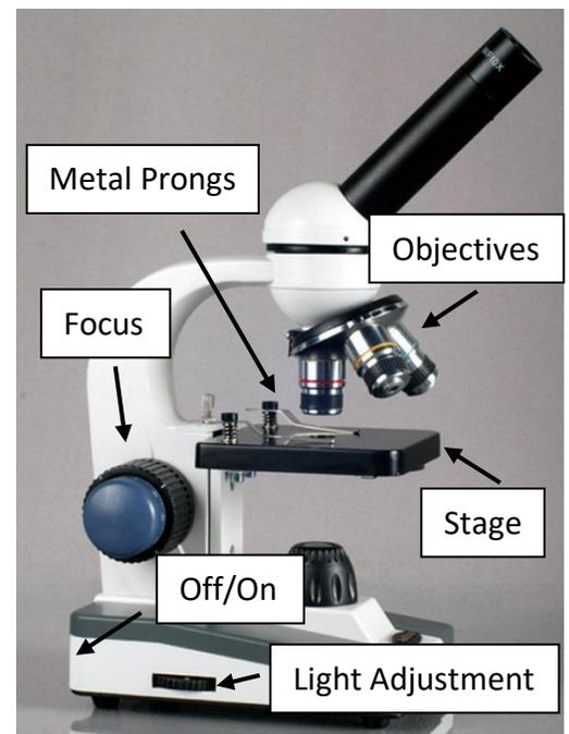
(100X magnification). While looking through the eye piece, adjust the focus using the large knobs on the sides. Refer to the 1-page Microscope User Manual for more information.
