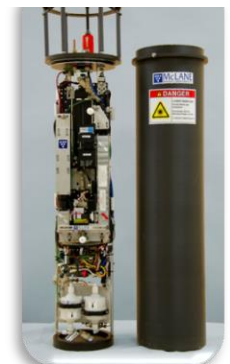
IFCB is an instrument that uses video technology to capture plankton images.
