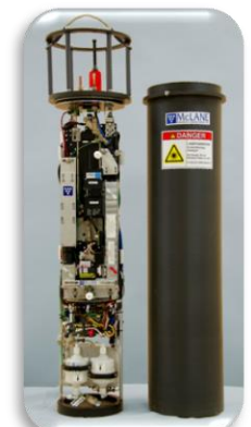
IFCB is an instrument that uses video technology to capture plankton images.
