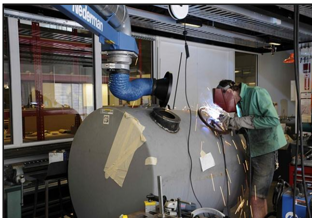
Figure 14. Welding the handle onto the anaerobic digester. http://parksparkproject.com
