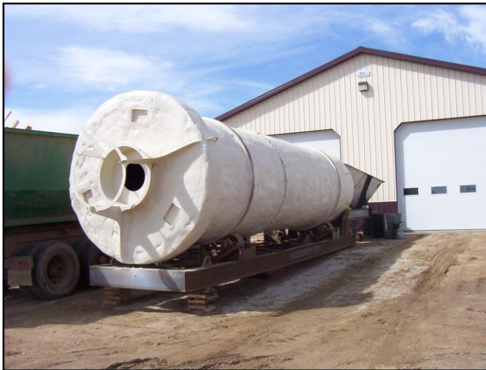
Figure 17. In-vessel tumbler that will be used for dog waste composting trials in the near future. Photo courtesy of EnviroWagg.
