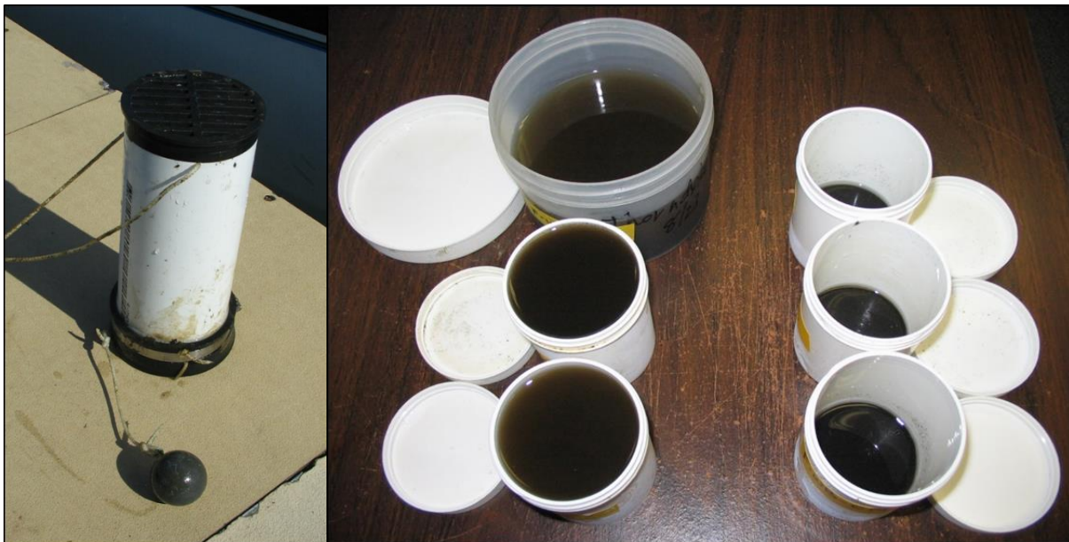
Figure 23. Biodeposit collection unit (left) and transferred deposits (right).
