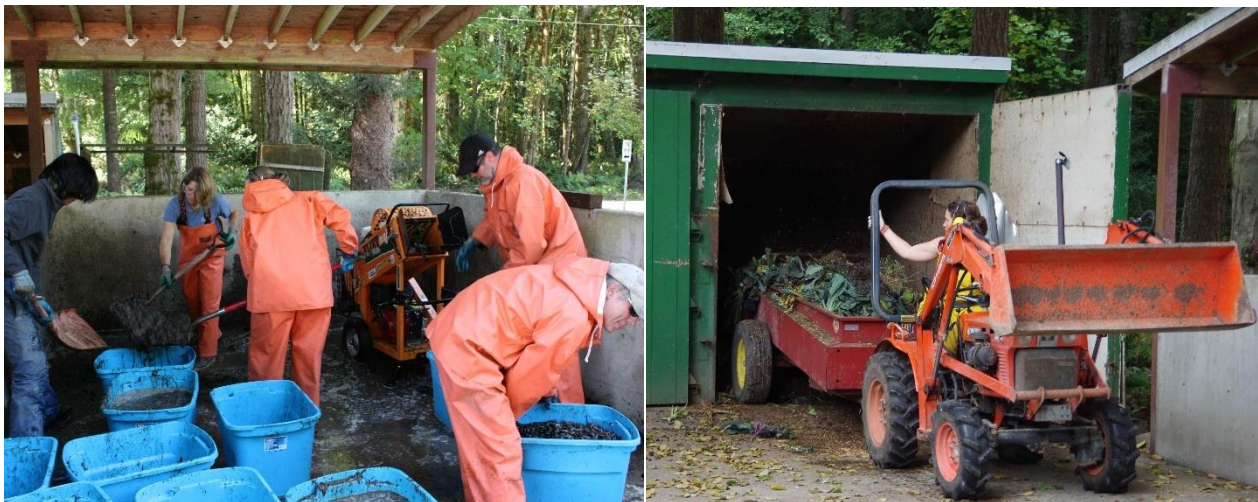
Figure 50. Chipping mussels (left) and loading mussels and green waste into the "reactor" (right) at TESC.
