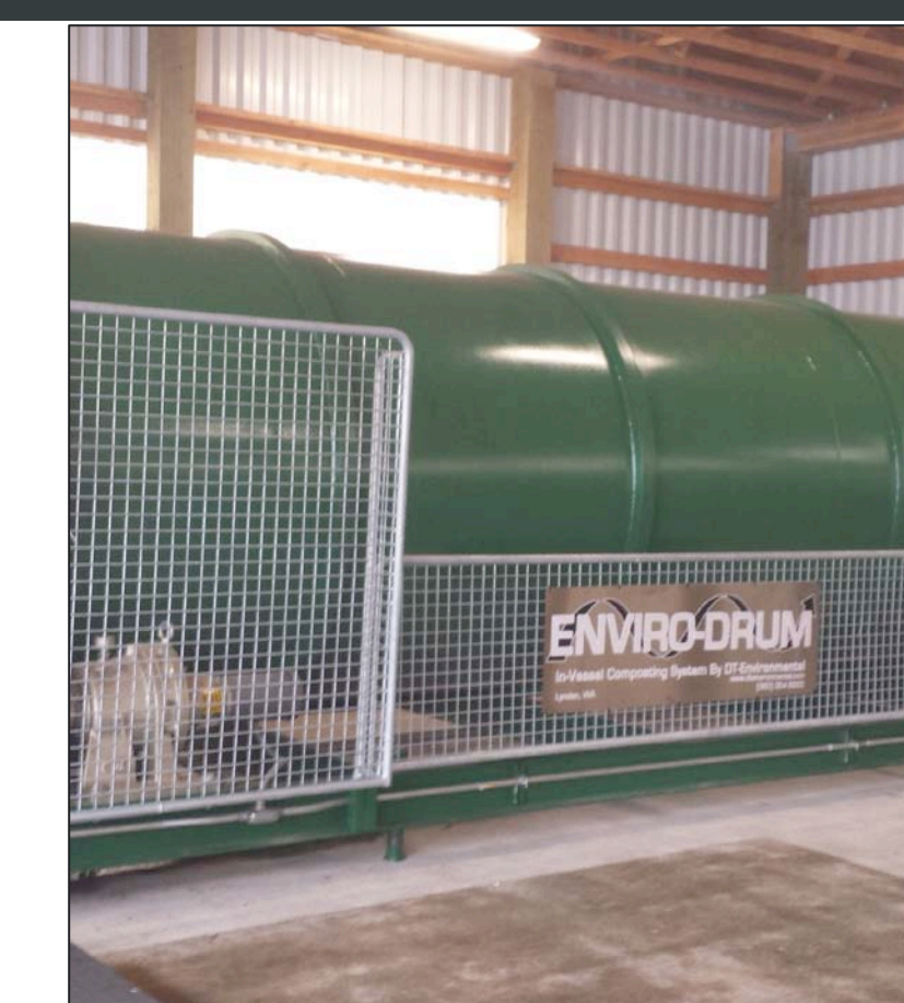
Figure 4. Mussels were mixed with other materials at the Washington Corrections Center for Women using their Enviro-Drum for composting
